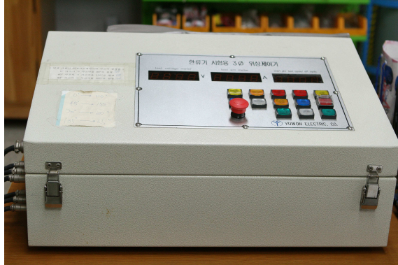
Fig. 20. The phase controller for various fault simulation
