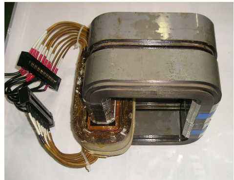
Fig. 14. A designed reactor for the transformer of a SFCL
