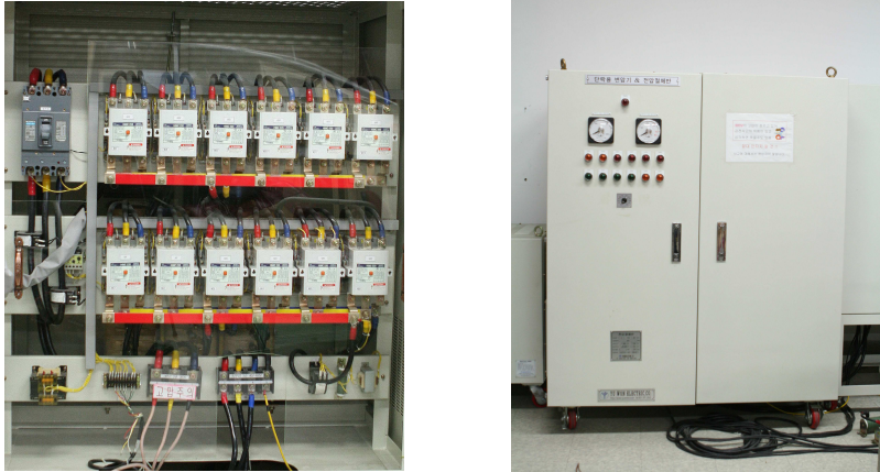
Fig. 18. The power system for various fault simulation
