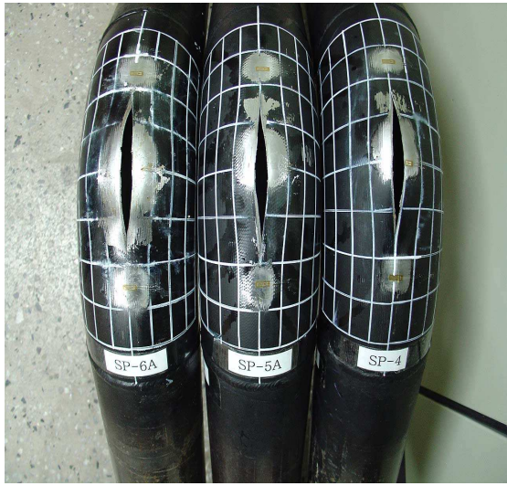
a) Extrados defect : \Theta/\pi = 0.125 \sim 0.5 b) Intrados defect : \Theta/\pi = 0.125 \sim 0.5
