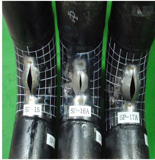
a) Extrados defect : \Theta/\pi = 0.125 \sim 0.5 b) Intrados defect : \Theta/\pi = 0.125 \sim 0.5
