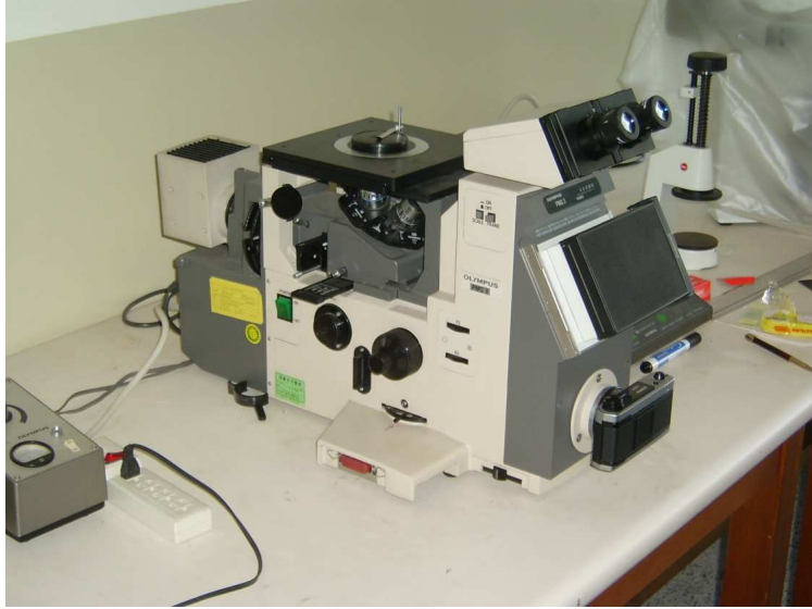
Photo. 3.1 Optical microscope for the micro structure test
