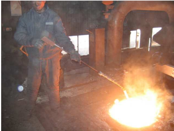
Fig. 3.10 Temperature check to the out of melting
