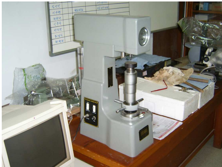
Photo. 3.2 Brinell hardness test machine
