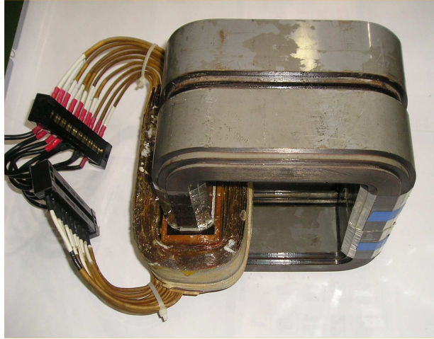
Fig. 11. The appearance of the designed reactor
