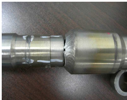
Fig. 4-3. Toe failure of socket welded pipe specimens
