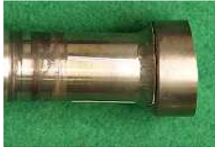
Fig. 4-4. Root failure of socket welded pipe specimens
