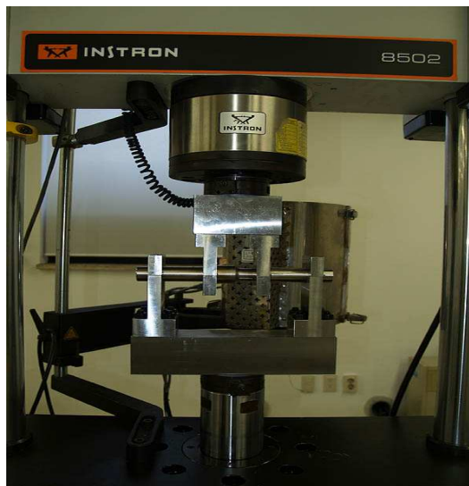
Fig. 3-1 4-point bending fatigue tester
