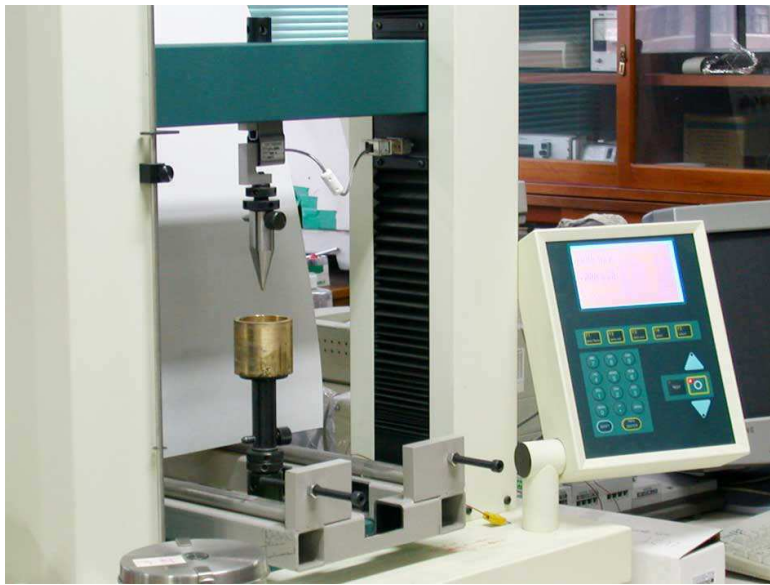
Fig. 3. 2 Photograph of compression tester with hot and cold bath.
