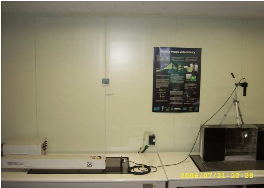
Photo. 1 Experimental equipments of PIV and test duct
