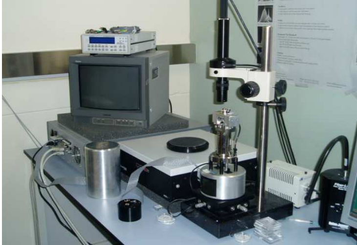
Photo. 3.3 Atomic force microscope
