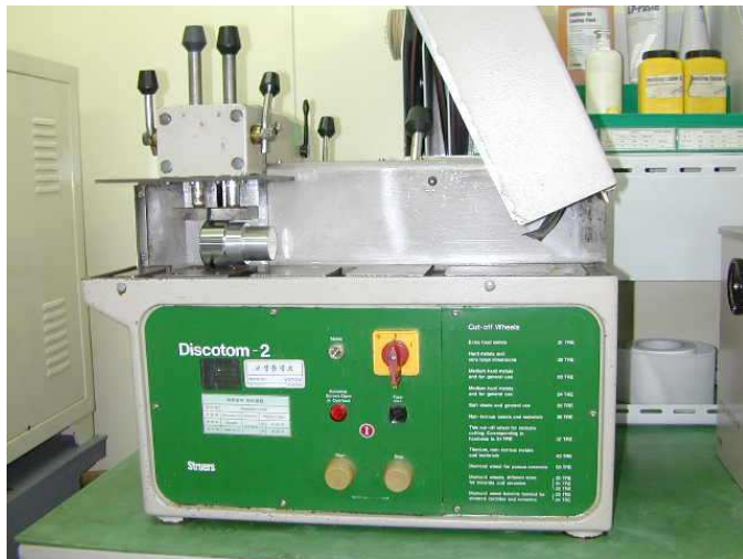
Photo. 3.4 Abrasive cutting machine
