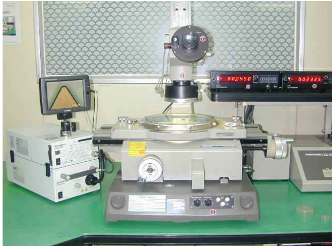
Photo. 3.6 Tool maker's microscope
