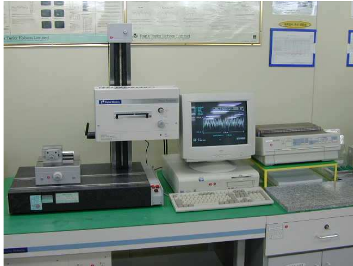
Photo. 3.2 Surface roughness tester
