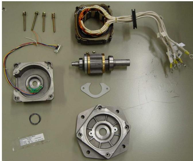
Fig. 5-1 Exploded view of 8/6 SRM
