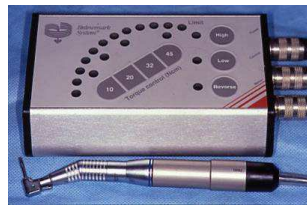
b: electronic torque controller
