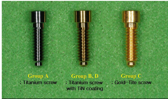
Fig. 1. Kinds of abutment screws
