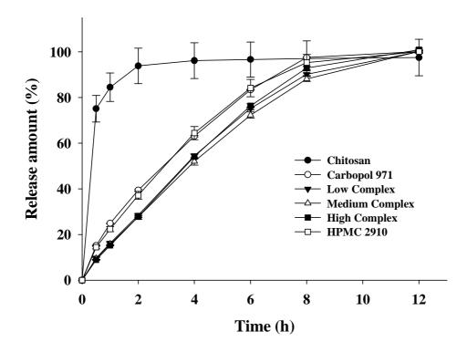
**Fig. 5.** Release profiles of theophylline from the tablets consisting of various excipients in pH 1.2.
