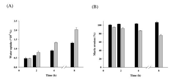
**Fig. 7.** Water uptake (A) and matrix erosion (B) of tablet containing 250mg chitosan/Carbopol interpolymer complex (IPC) in pH 1.2 (gray column) and 6.8 buffer (black column).
