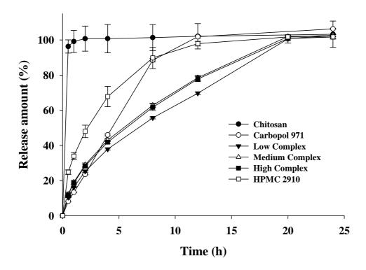
**Fig. 4.** Release profiles of theophylline from the tablets consisting of various excipients in pH 6.8.
