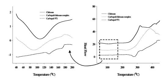
Fig. 2. Comparison of the DSC thermogram of the chitosan/Carbopol interpolymer complex (IPC) with those of chitosan and Carbopol.
