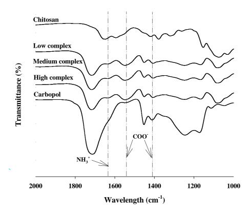
Fig. 1. FT-IR spectra of chitosan, Carbopol and chitosan/Carbopol interpolymer complexes (IPC) with various molecular weight of chitosan
