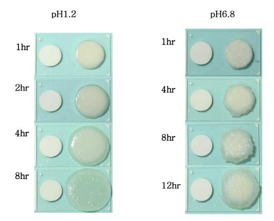
**Fig. 6.** Effect of the pH of the medium on the swelling and dissolution of the theophylline tablet containing chitosan/Carbopol interpolymer complex
