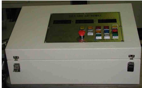
Fig. 20. The phase controller for fault simulation
