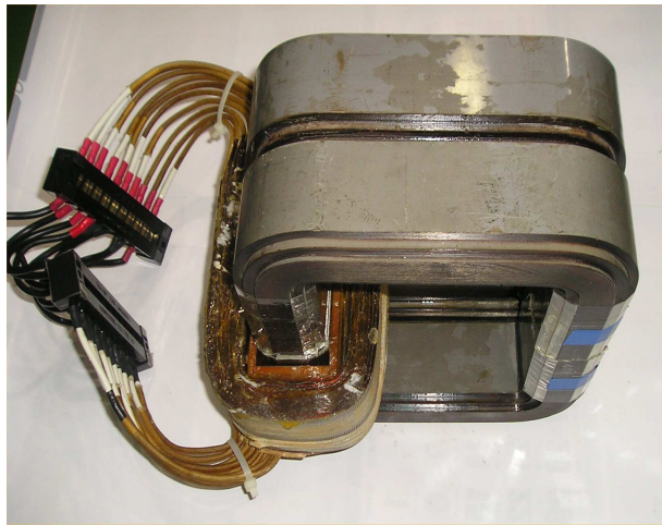
Fig. 15. The appearance of the designed reactor
