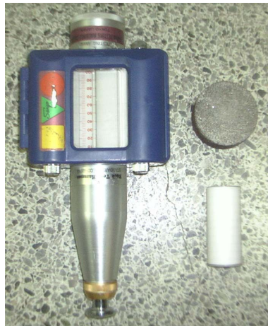
Figure 5.17. Photograph of the Schmidt hammer test.
