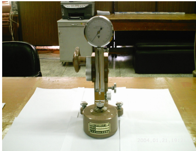
Figure 5.14. Photograph of Shore Scleroscope Hardness tester.
