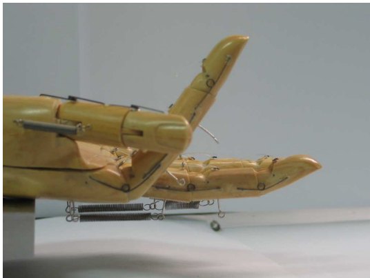
Fig. 5-14 Shape of 3rd Joint for the Number of Segmented SMA wire
