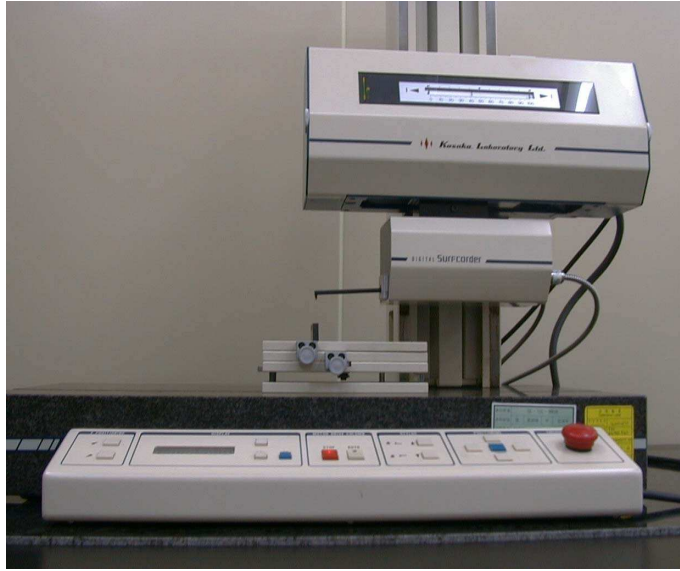
Photo. 3.2 Surface roughness testing system
