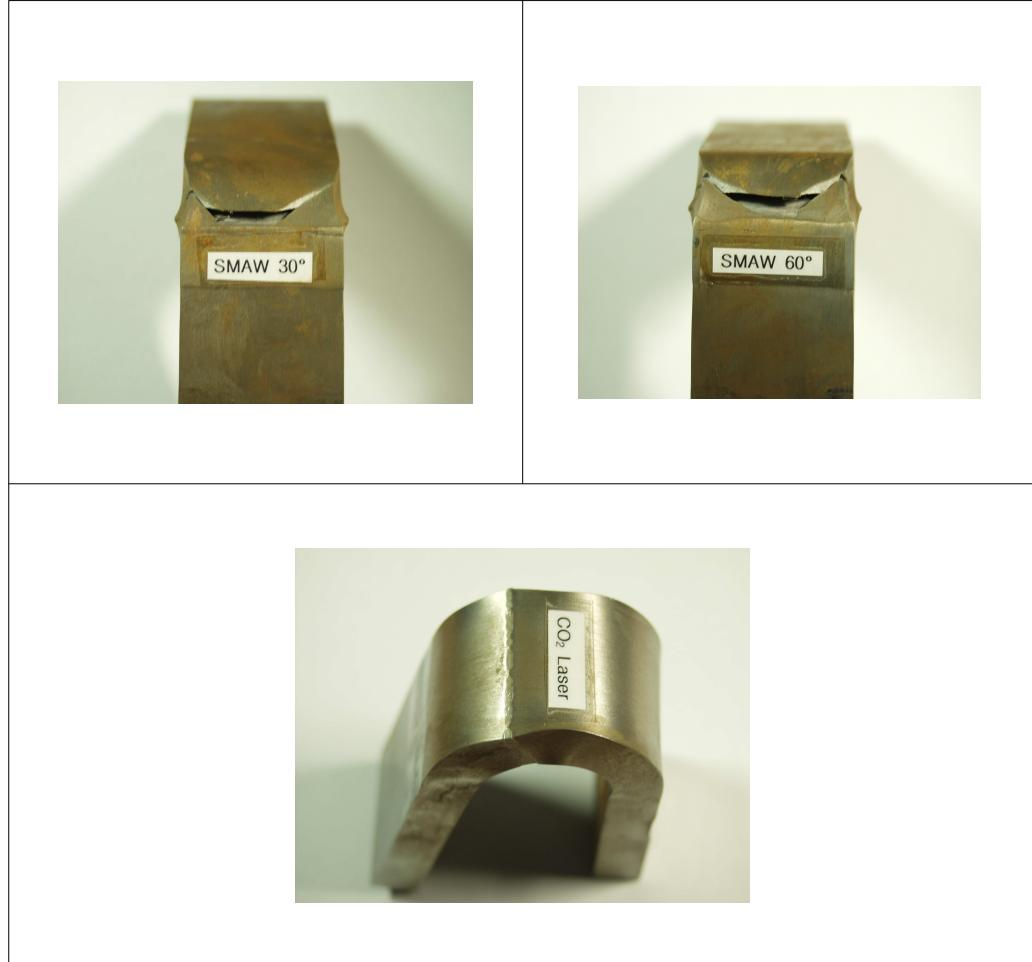
**Fig. 18 Results of Bending Test**
