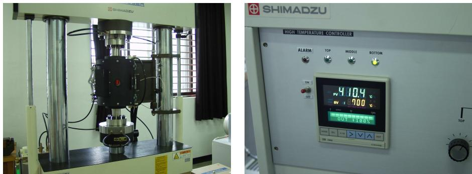
**Fig. 21 Machine of High Temperature Tensile Test**
