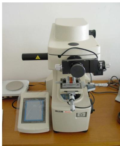
Fig. 13 Micro Vickers Hardness Tester
