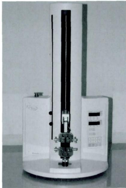
Figure 2. EZ test for microtensile
