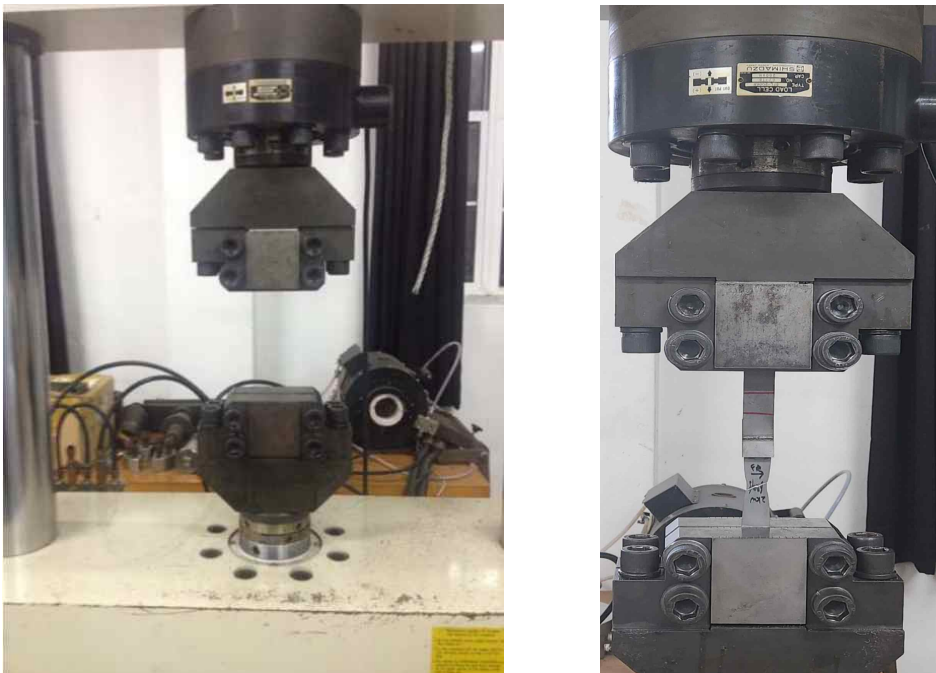
Fig. 3.3 Process of shear test
