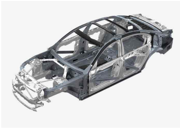
Fig. 1.4 BIW(Body in white) of company B with CFRP applied
