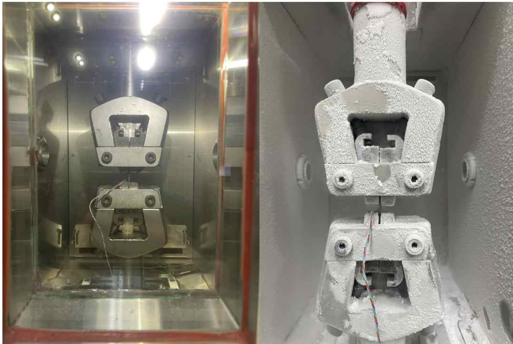
Fig. 3. 4. Tensile test in cryogenic environments.
