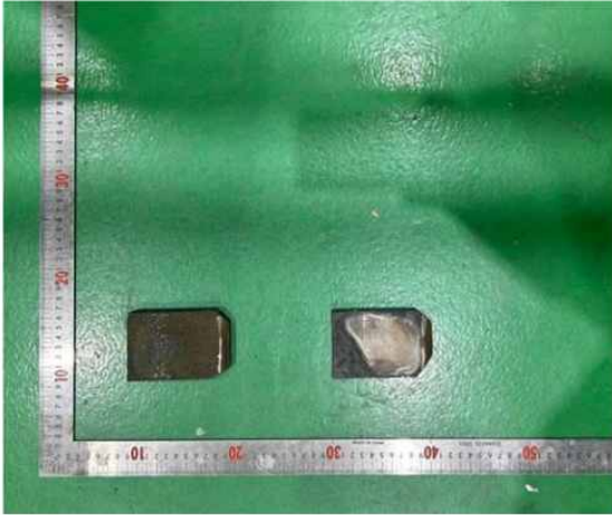
Fig. 3. 1. Test specimen before and after hot rolling and cold rolling.
