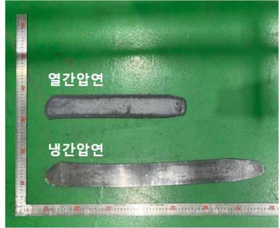
Fig. 3. 1. Test specimen before and after hot rolling and cold rolling.
