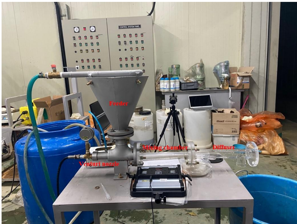
Figure 2.6. Measurement of bubble size using high speed camera
