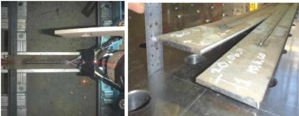
Fig. 1.2 Experimental set up and test specimen for heat sink welding(Liquid CO<sub>2</sub>)
