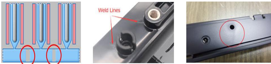
Fig. 1.2 'Weld line' defect generated in multi-component injection molding
