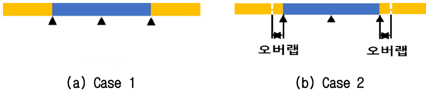
Fig. 2.9 The opening time of the secondary gates before(a) and after(b) applying overlap molding technology
