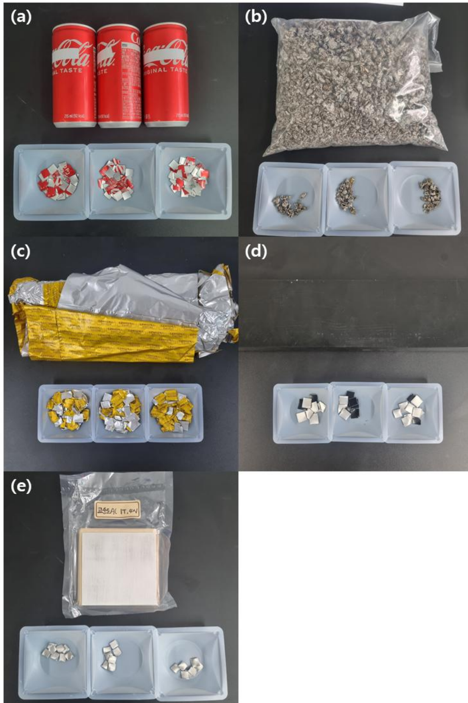
Figure 3-2. Aluminum samples used in aluminum hydration reaction, (a) Used beverage cans (A3104), (b) De-coated Al can granules (A3104, A5182), (c) Construction Al materials (A6063), (d) Yogurt lids (A8011), (e) High-purity Al (99.99%)
