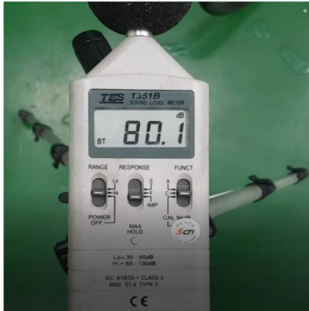
Fig. 4-6 Noise Test Measurement (21T)
