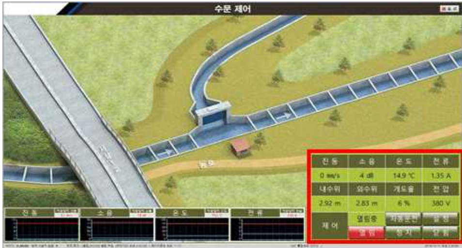
Fig. 3-27 Program screen when water gate is opened
