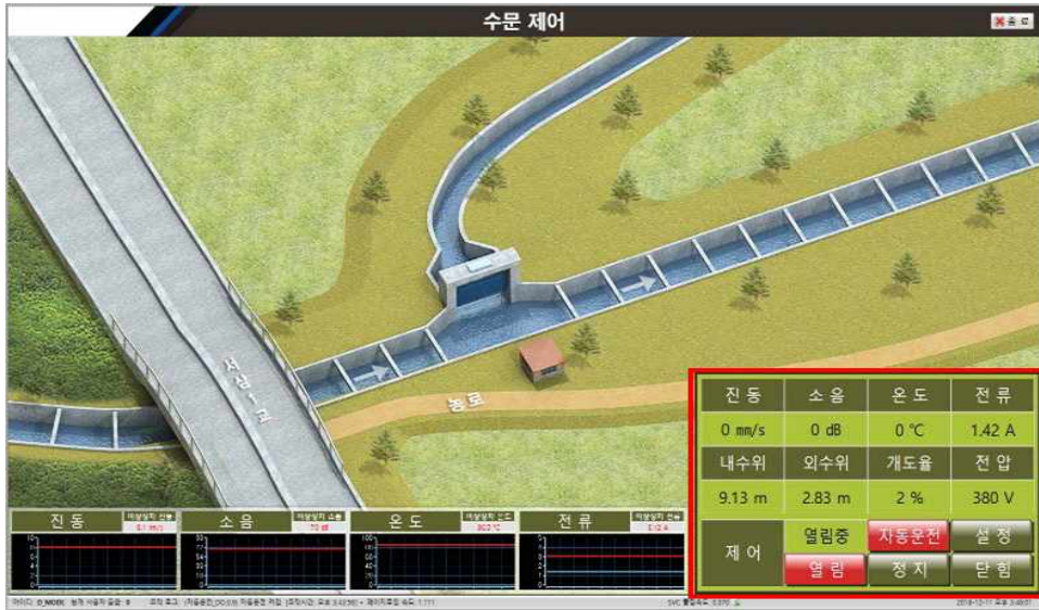
Fig. 3-77 Program screen when water gate is opened
