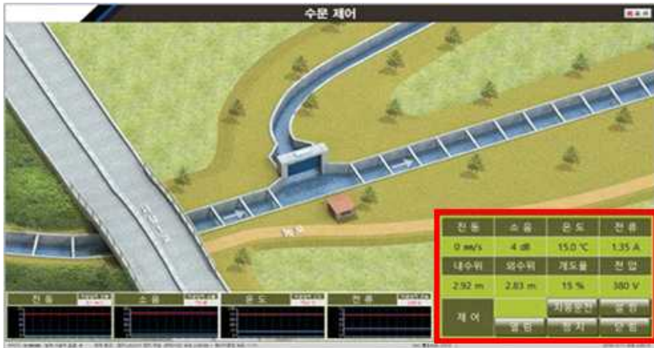
Fig. 3-30 Status program screen before full closing of the water gate
