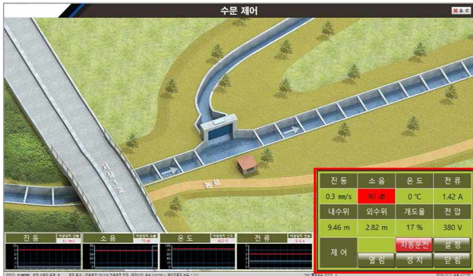
Fig. 3-90 Change the color of the noise display on the program screen and stop the water gate
