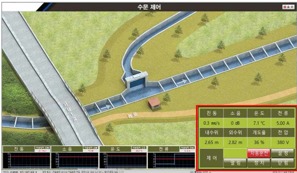
Fig. 3-96 Program screen where the sluice gate is stopped by exceeding the set current value
