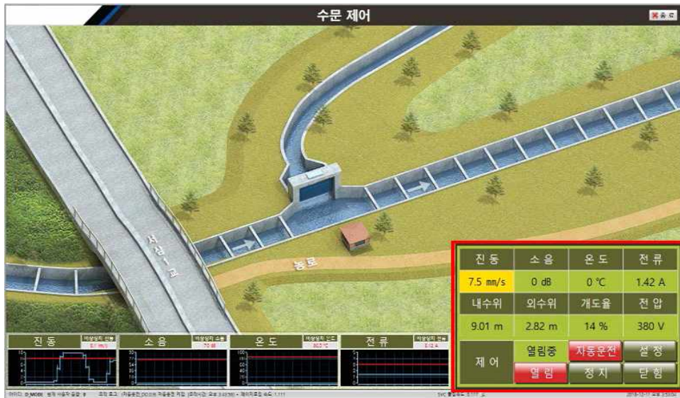
Fig. 3-80 Change the color of the vibration display when the water gate is opened
