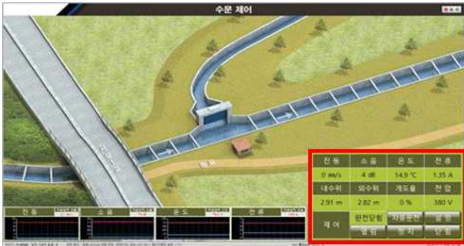
Fig. 3-32 Status program screen when the water gate is completely closed
