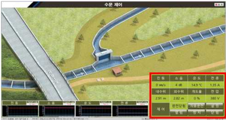
Fig. 3-35 Program screen before click to gate opening
