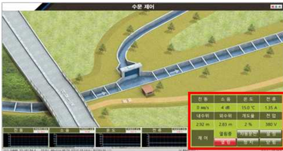
Fig. 3-38 Program screen after clicking to open the water gate
