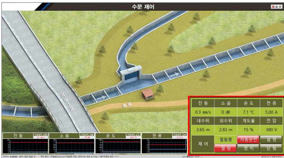
Fig. 3-98 Program screen when water gate is opened
