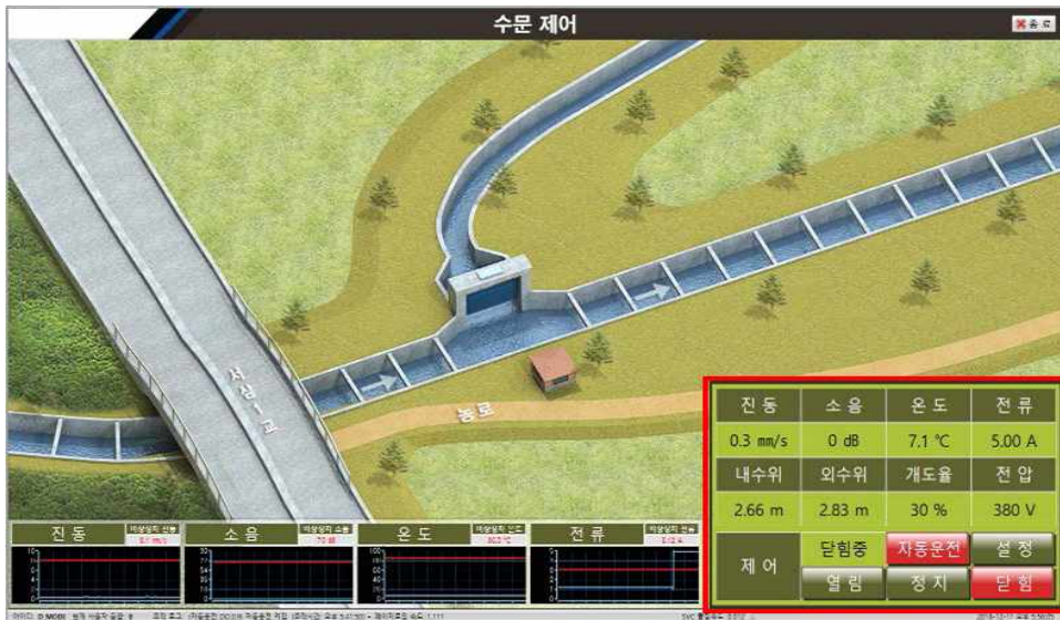
Fig. 3-93 Water gate closing program screen
