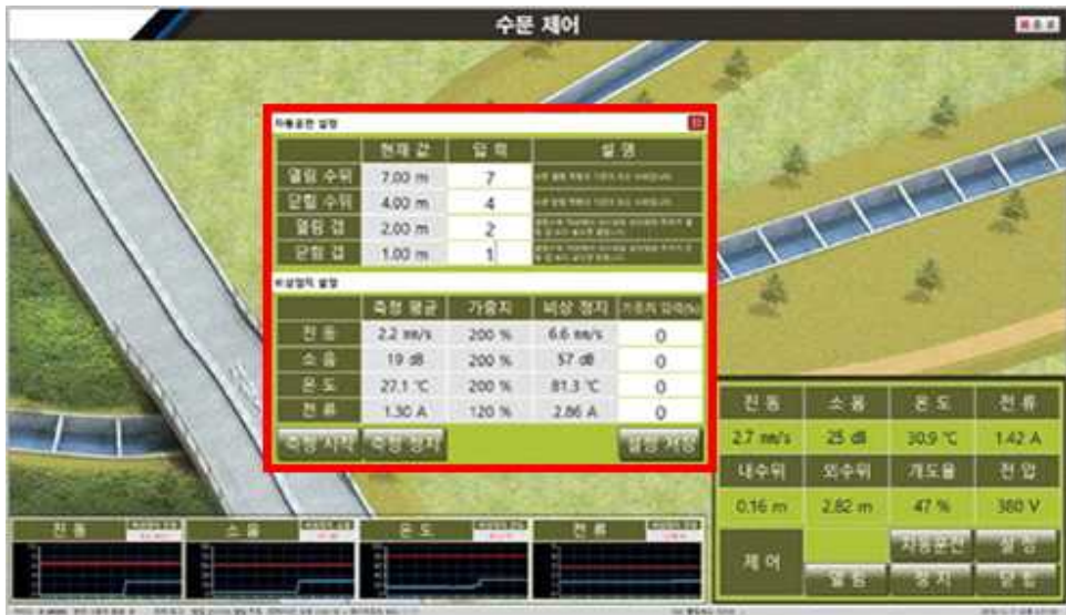
Fig. 3-74 Water level setting and measurement program screen
