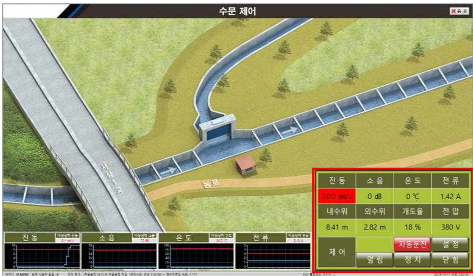
Fig. 3-82 Change the color of the vibration display part of the program screen and stop the water gate
