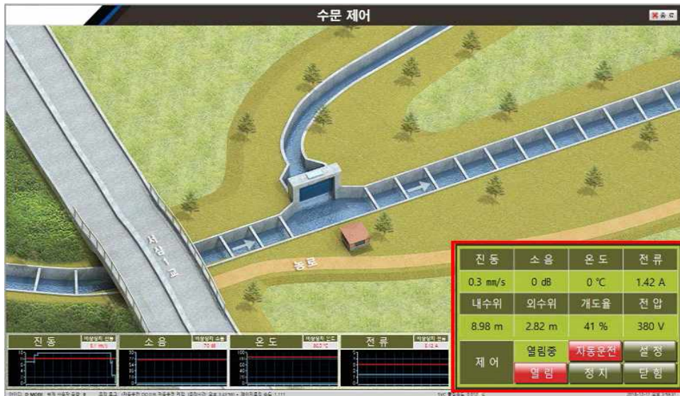
Fig. 3-84 Change the color of the vibration display when the water gate is opened
