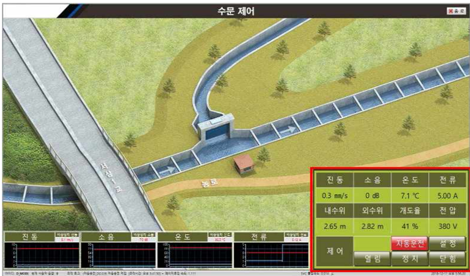
Fig. 3-100 Program screen when the water gate is stopped
