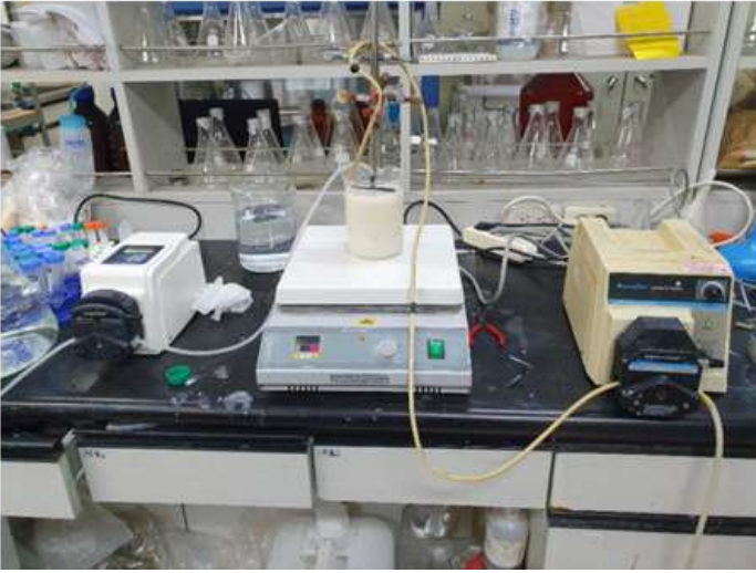
Figure 3.2. Schematic diagram of (a) experimental setup and image of (b) experimental setup and (c) functional ceramic membrane module.
