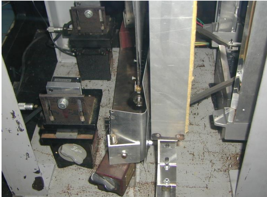
Fig. 5.13 Setup of heaters and insulation plates
