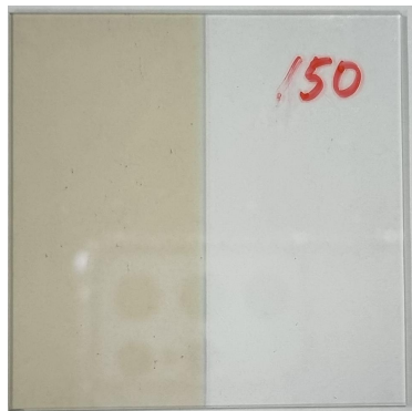
Fig. 3-5 ITO Specimen with Sputtering Method
