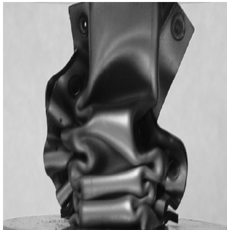
Photo. 12 Crush pattern after axial static test on STD specimen
