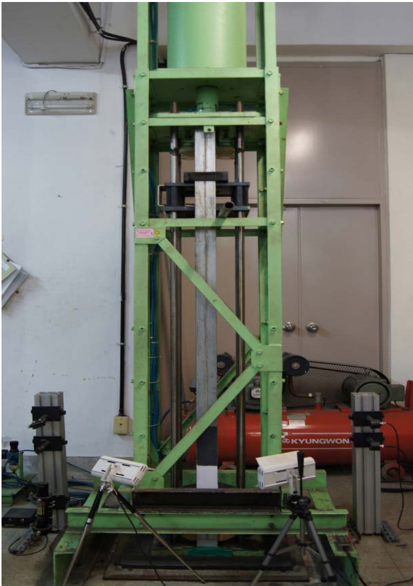
Photo. 3 Impact testing setup for curshing 20)
