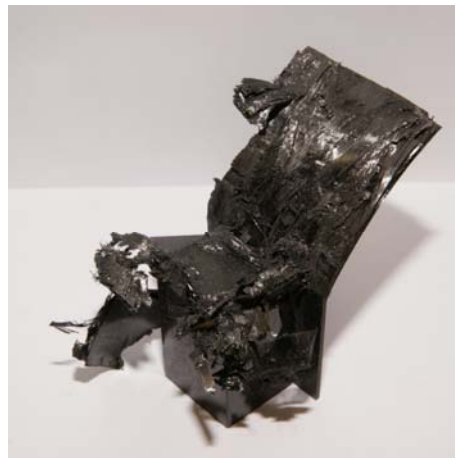
Photo. 6 Shape of collapsed CFRP single hat shaped member 35)
