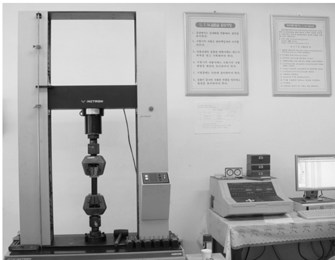
Photo. 2 Equipment for static tests (UTM).
