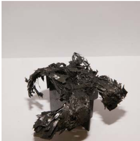
Photo. 8 Shape of collapsed CFRP double hat shaped member 35)
