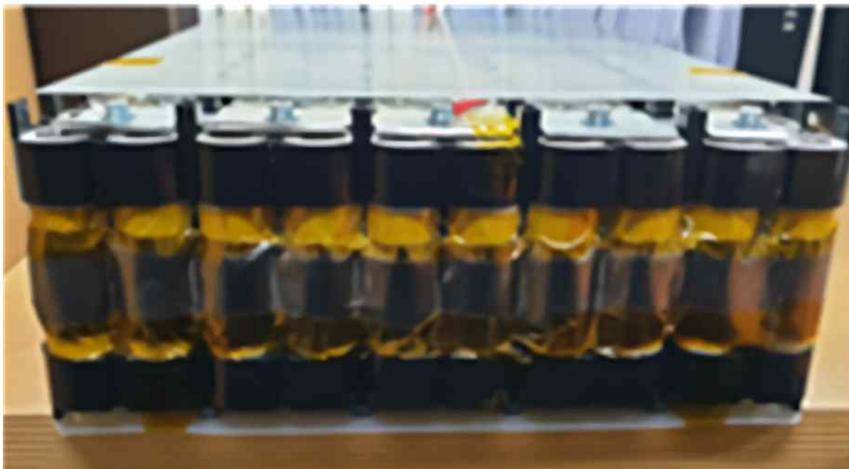
Fig. 3-5 Electronic Device Application of Graphite Sheet
