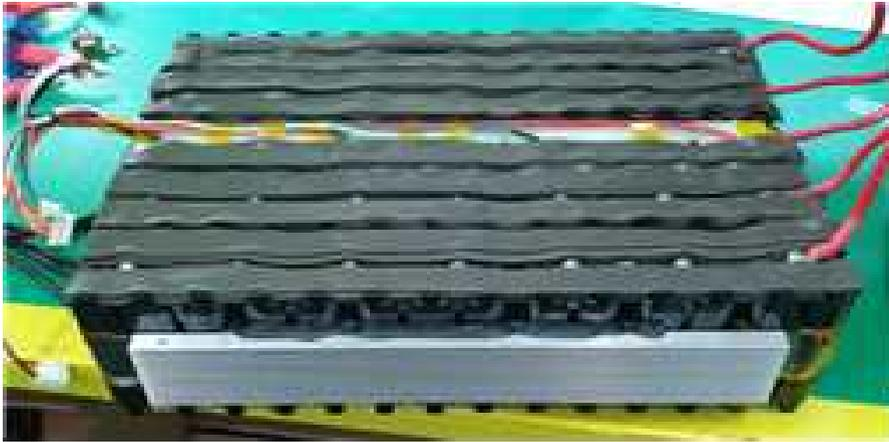
Fig. 3-6 Electronic Device Application of Silicone Sheet
