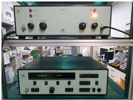
A. Power amplifier Type 2712, Sine generator Type 1051
