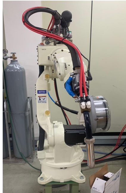
Fig. 2.2 AC pulse MIG welding machine and 6 axis welding robot
