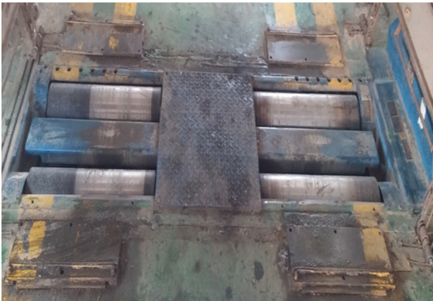
Fig. 14 Photograph of chassis dynamometer measurement equipment
