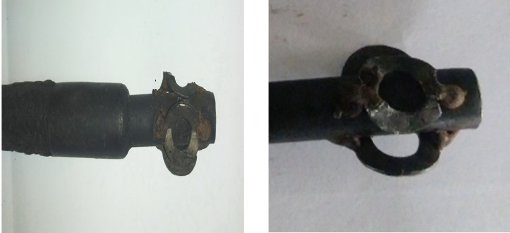
Fig. 7 Shape of damaged smoke measurement probe(A)
