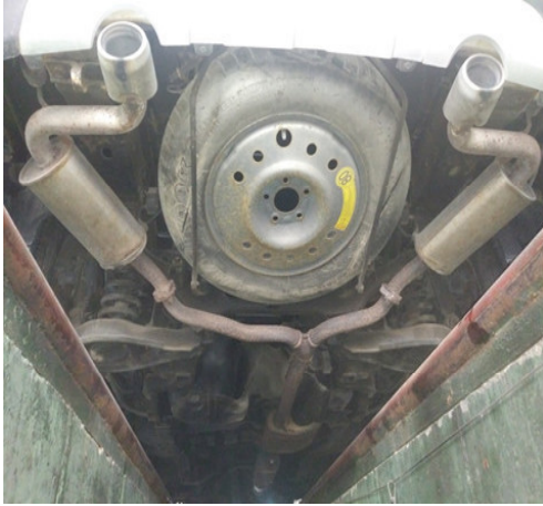
(a) Small exhaust pipe
