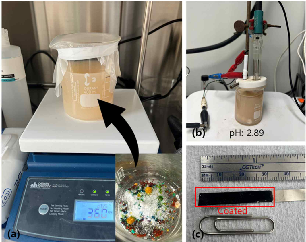
Fig. 4-5 Manufacturing process of super-hydrophilic surface: (a) Solution preparation (b) ECD (c) Super-hydrophilic surface formation.
