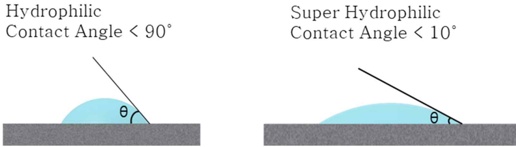
Fig. 2-2 Contact angle range of hydrophilic and super-hydrophilic.
