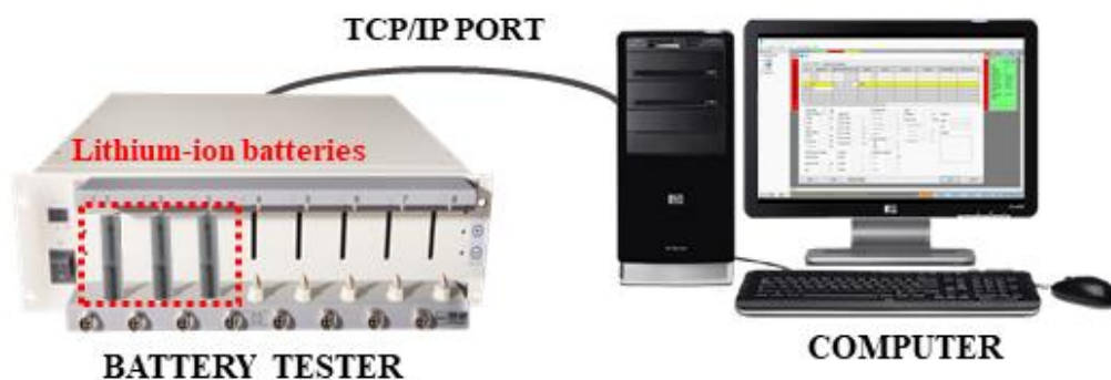
Fig. 2.1 Battery charging and discharging experimental setup
