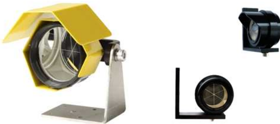
(a) Large Monitoring Prism
