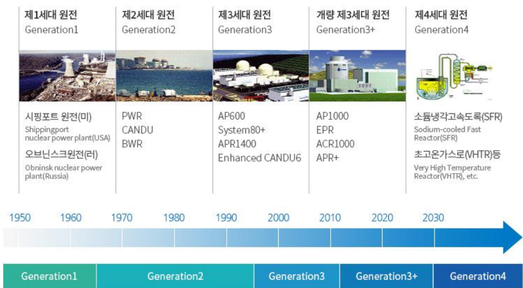
Fig. 1.4 Diagram of the nuclear power generation [13]
