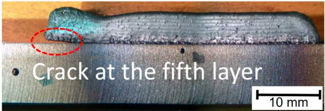
Fig. 2 Defects of products manufactured by the metal AM Process 43)
