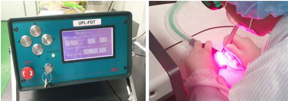
Fig. 2. A diode laser(660nm red light) is irradiated onto the tumor of the SCID/ICR mouse.
