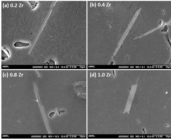
Fig. 4. 4. SEM observation of (Al,Si)_3(Ti,Zr)
