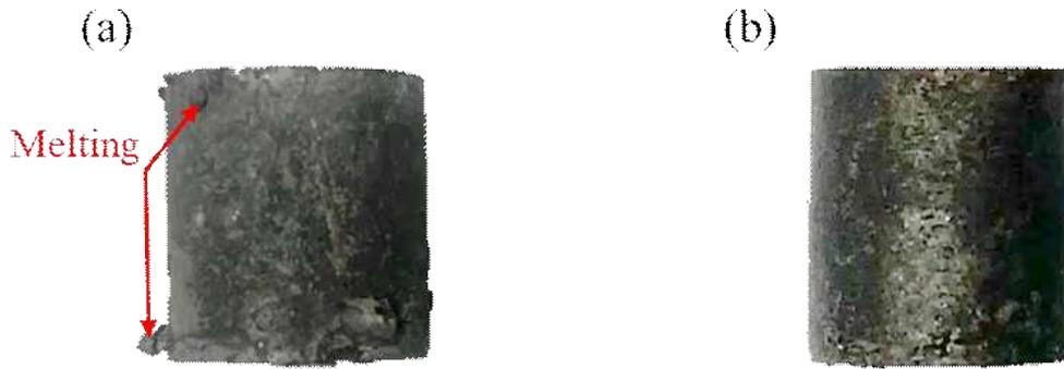
Fig. 56. Appearances of the specimens at the test temperature of 1100°C according to the heating temperature of (a) 1200°C and (b) 1100°C.
