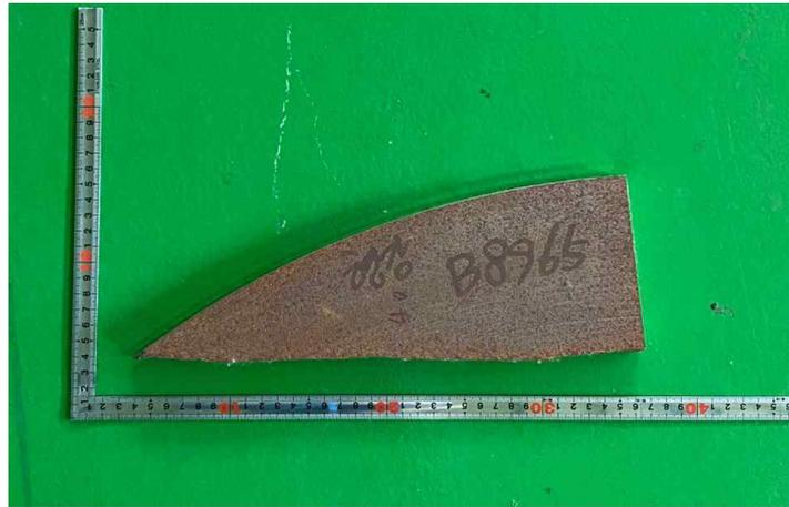
Fig. 16. The as-received adamite cast steel.
