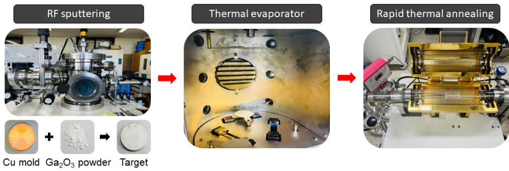
Fig. 11 Experimental equipment of rf sputtering, thermal evaporator, and rapid thermal annealing in order, respectively.
