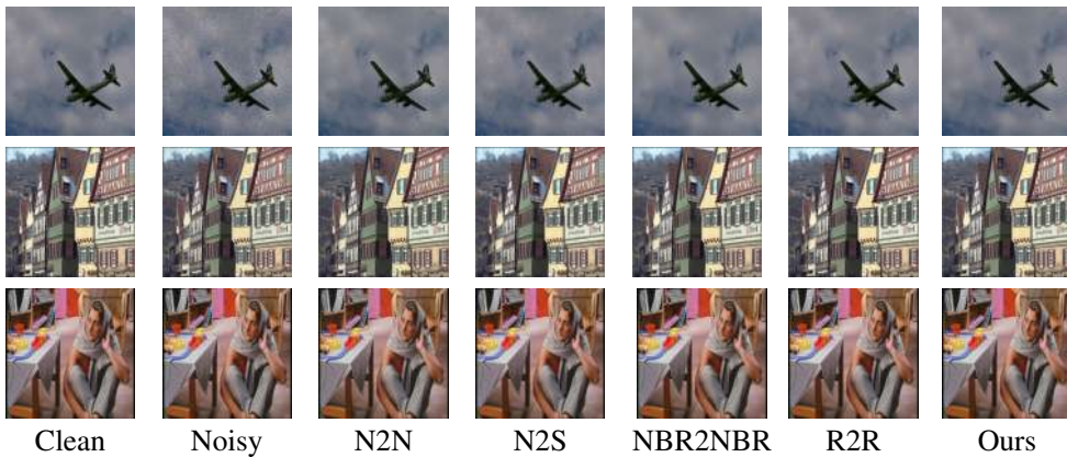
Figure 6: Visual comparison of the results from different methods when the denoising images recorruped by Poisson \lambda = 30 . The three images of the three columns are adopted from BSD68, Kodak24, and Set14 respectively.
