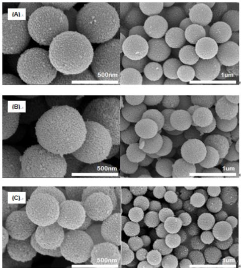
Figure 3. SEM micrographs of TiO<sub>2</sub> powder prepared by hydrothermal reaction methods at the different temperature (TTIP:H<sub>2</sub>O ratio=1:6, 5 h) (A) 110°C, (B) 150°C and (C) 190°C.
