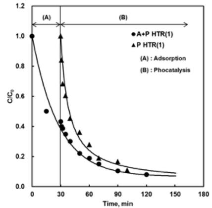
(a) Variation of MB concentration as a function of time in A+P and P systems over HTR(1)
