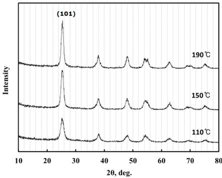
Figure 2. XRD pattern of different size TiO<sub>2</sub> spheres prepared by hydrothermal reaction at 110, 150 and 190°C for 5 h.
