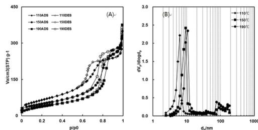
Figure 1. Nitrogen adsorption–desorption isotherms (A) and the corresponding pore size distribution curves (B) of the porous TiO<sub>2</sub> microspheres prepared at different temperatures for 5 h: 110, 150 and 190 °C.
