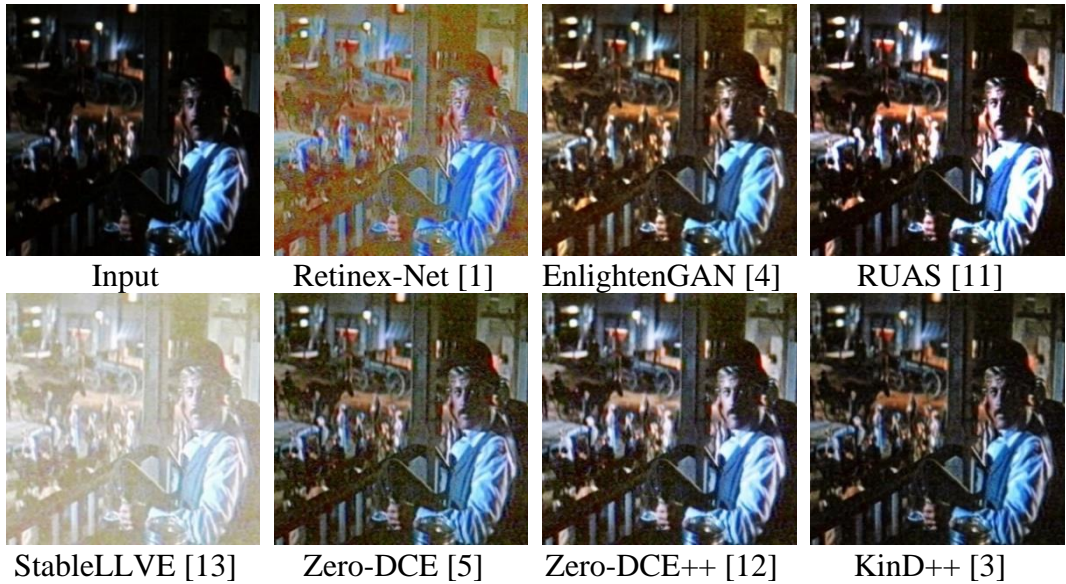
Figure 1-3. Visual comparisons of brightness enhancement for old video frames using state-of-the-art methods: Retinex-Net [1], EnlightenGAN [4], RUAS [11], StableLLVE [13], Zero-DCE [5], Zero-DCE++ [12], and KinD++ [3].
