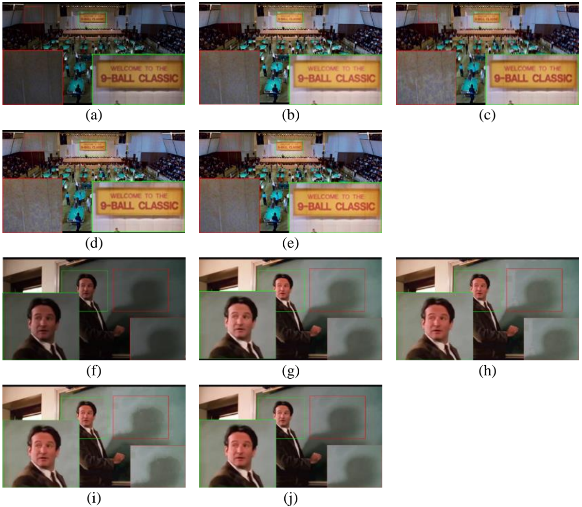
Figure 4-2. Ablation study: (a) Input Image, (b) Only DCE-Net, (c) Only illumination Network without any attention module, (d) DCE-Net with illumination network without any attention module, (e) Curve estimation network with attention-based illumination network (proposed) and the same for (f), (g), (h), (i), (j), respectively.
