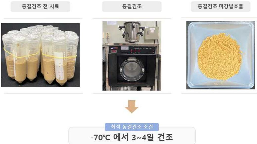
Figure 2. Freeze drying conditions of fermented rice bran
