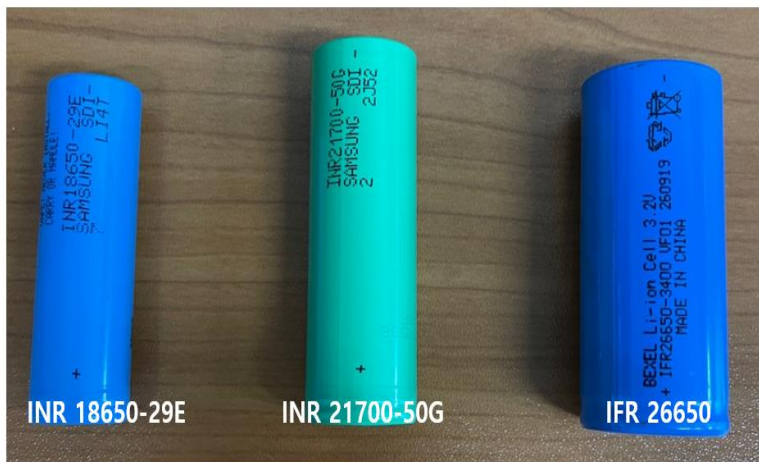
Figure 16. Cylindrical battery cells used in the experiment
