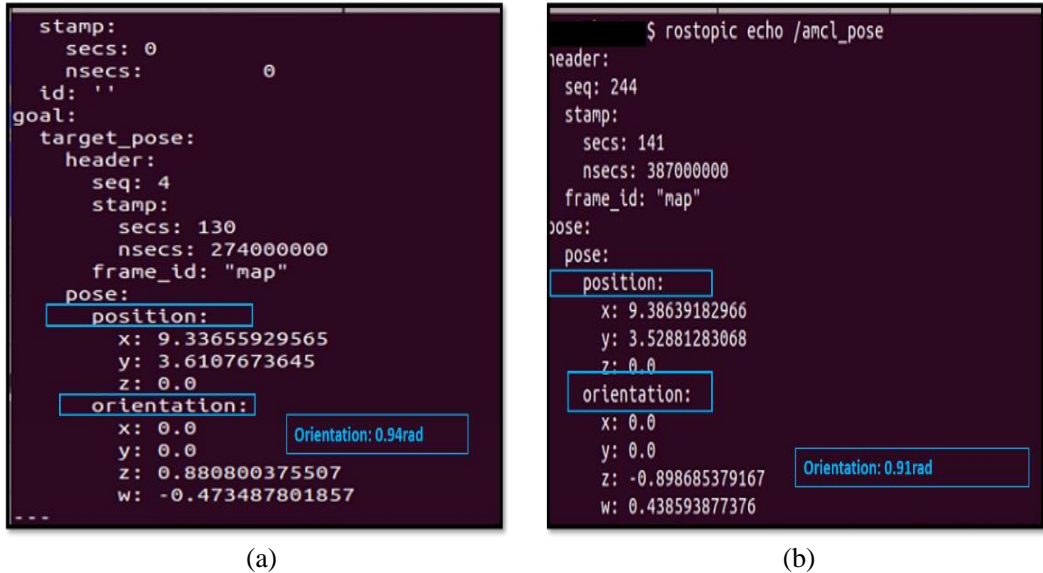
Figure 5-11 The target position and orientation (a) and the estimated pose (b) of the robot in Figure 5.10
