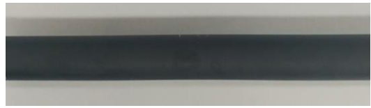
(a2) Surface absorption receiver tube (Copper tube coated with graphite)
